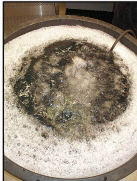
Figure 8. Wash tub with air hose to produce foaming action.
