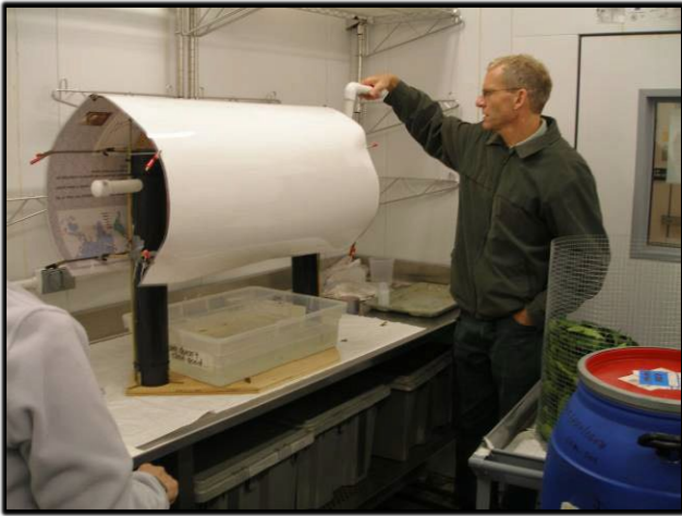
Figure 5. Raffle drum with shield to direct falling debris.
